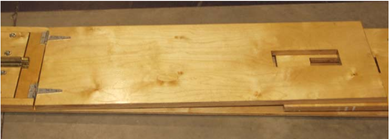
Section 1 — bottom view — legs folded — note: longer leg should be down first.
