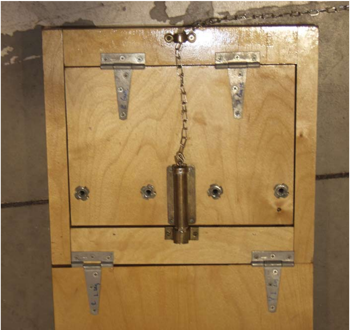
Section 1 — bottom view — starting gate
