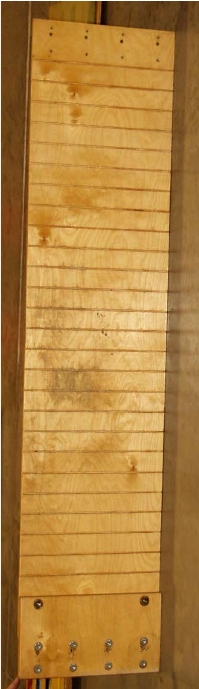
Section 2 — bottom view — showing kerfs
